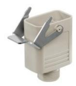
Housing in plastic or metal version. For power supply in the smallest possible space; neck for cable gland integrated, use with special H-Q cable glands; with mnetal housing EMC cable gland as an option
