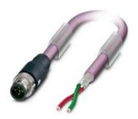
Robust, pre-assembled PROFIBUS M12 (B-coded) cable with PUR (halogen-free) outer sheath for flexible use (drag chain). Shielded version.
