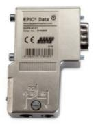
Data Connectors D-Sub (9-pin.) For PROFIBUS DP according to IEC 61158, IEC 61784, with spring type (ST) connection, 90 ° cable outlet and PG (option)
