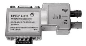
Data Connector D-Sub (9-pin.) for PROFIBUS DP according to IEC 61158, IEC 61784, with optical interface and repeater functionality and optical fiber interface (POF and PCF)
