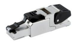
RJ45 field mountable Industrial Ethernet connector, IP20; qualified for 10 Gbit data transmission, acc. to TIA568 A; with metal housing, for industrial environment
