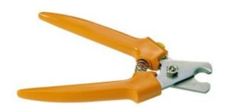
Cutting tools/cable shears for small fine-wire conductors up to an outer diameter of 11 mm, Semi-circular cutting edges prevent cable from being deformed
