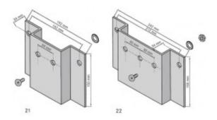
MP 21/22 installation sheets for all round and large flat cables wedges
